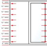
F. **Doors using Installation Clips:** Install installation clips. Place the clip so that the lip is facing up and against the flush flange, at the locations shown in the placement diagram. Secure the clip by driving #6 x 5/8" corrosion resistant screws through the outer two holes of the three holes shown.
